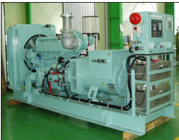
Emergency Generator Set (150kW, 60Hz)
